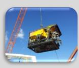
The work included flange installations, flying leads replacement, cable detection surveys, sub-sea trees installation, acoustic transponders installation and retrieval and various survey/inspections
